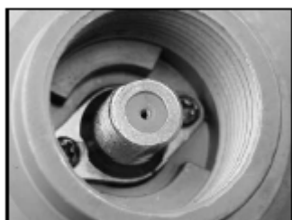
Figure 3 Antenna mast socket with type F connector
